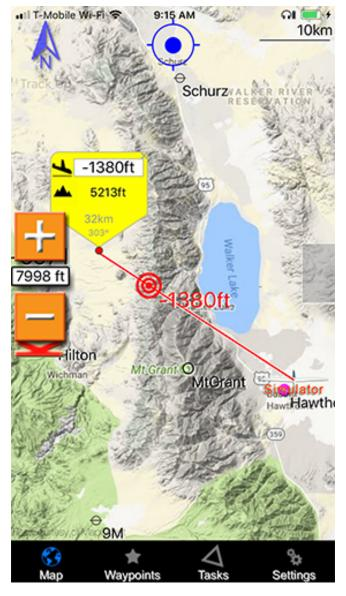
DEM waypoints can also be used in the Simulator. The location of simulated glider can be easily changed by dragging the glider symbol on the map to the desired location. When dragging the glider, a plus and minus buttons appear, which allow changing of the simulated glider's altitude (see left).
