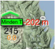
In the example above, the regular final glide calculator shows that the task destination (Minden) can be reached at 215m. However, the final glide over terrain calculator detected that the projected descent path will intersect the terrain to the depth of 202m. Therefore, to reach the goal, the pilot must climb at least 202m higher, plus any safety buffer for the errors in terrain database, and any other factors that the pilot should take into account.
