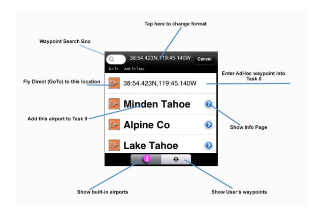
2. Tap the image (not the text with coordinates) on the first entry in the dialog. This will create an Ad Hoc waypoint at the tapped location and engage the Direct To, or Go To function to the selected location. If you want to edit or fine tune the location, tap at the end of the blue goto line to see the blue edit location circle:
